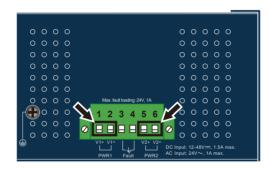
Figure 3-1: IGS-4215-16T2S Inlet Power Socket
